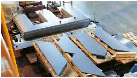
Transformer Core Rated Power 20 MVA
