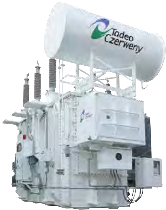
Rated Power: 25/40 MVA, Ratio: 138 ( \pm 4 \times 2,5\% NLTC) & ( \pm 16 \times 0,625\% OLTC) / 25 kV Tertiary (13.8 kV): Not accessible Frequency: 60 Hz; Weight: 85 tn; Client: ENELDIS (Venezuela)
