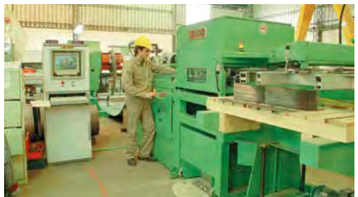
Automatic core cut line STEP LAP Type
