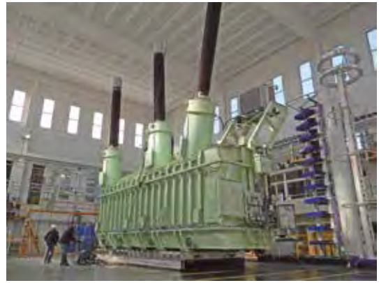
Fully equipped HV Laboratory, to test up to 550 kV transformers
