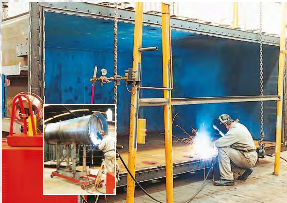
Transformer Tank Rated Power 30 MVA.
