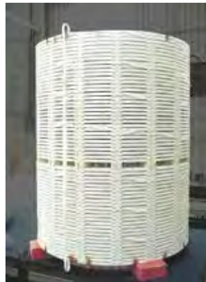
Continuous Interleaved Dis Winding
